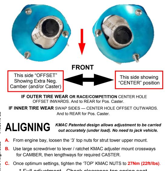
\* Full adjustment - Check clearance top spring seat to Inside of Strut tower on steering rotation
